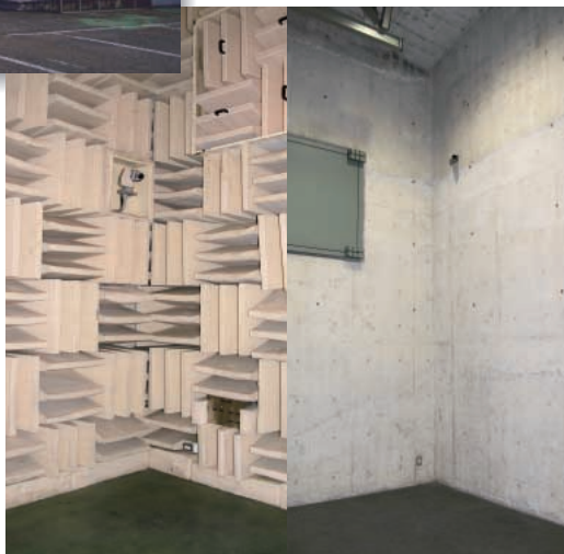
Insulated Acoustic Room (Semi-Anechoic Wall)
